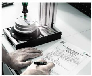
All Wera torque tools are produced, adjusted, calibrated and certified under strict quality conditions. On request, Wera can also issue a calibration certificate according to DAkkS guidelines in cooperation with an accredited specialist laboratory.
