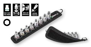
8-piece; robust textile socket belt, including snap hook to enable secure fastening to a belt loop or pocket. Non-woven reverse side and hook and loop strips for simple attachment e.g. to a wall, shelf, tool trolley and to the Wera 2go tool transport system. Fast and easy Twist to Unlock mechanism for secure storage and simple removal of the sockets.
