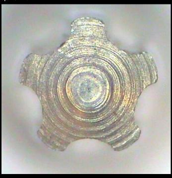
Standard drive bit production: underfilled and severe edge rounding minimises fit and performance.
