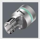
The clamping of the screw is achieved by two flexible locking balls and a robust, permanently elastic, heat-shrunk tubing. The tubing is effectively protected against mechanical wear and tear by a steel ring. The holding function is especially helpful in confined, hard-to-reach spaces, where there is no room for a second hand to secure the screw.
