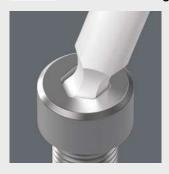
The spherical drive profile means that it is possible to swivel the axis of the tool to that of the screw, and therefore enable angled, "around-the-corner" screwdriving jobs.
