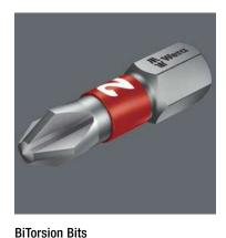
BiTorsion bits are absolutely premium products. They have a softer BiTorsion zone which reduces the hardness of the shaft in comparison to the drive tip. This means that the peak loads that cause bit breakage and premature wear are absorbed in this zone – something which enhances the service life of the bits.
