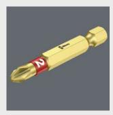
BDC-Bits are absolutely premium products. They have a softer BiTorsion zone which reduces the hardness of the shaft by about 20 % in comparison to the drive tip. This means that the peak loads that cause bit breakage and premature wear are absorbed in this zone — something which enhances the service life of the
