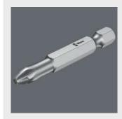
ACR® stands for "anti-cam-out ribs". ACR® bits have ribs at the drive tip that protect against slipping out of the screw head. It is recommended that ACR® bits are matched with ribbed ACR® screws for maximum effect. ACR® reg. trademark of Phillips Screw Company.
