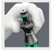
These torque screwdrivers are supplied with a fixed pre-set torque value. This is ideal for all applications that require constant, identical torque. They feature a pre-set torque range of 0.3 Nm to 4.0 Nm (adjustable between 0.3 Nm - 8.8 Nm), two different handles, measurement accuracy of  $\pm$  6 % and Rapidaptor chuck technology for rapid bit change.
