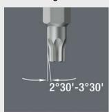
The conical TORX® profile provides a better fit in the screw. Combined with a great recess depth this produces a pinch effect.
